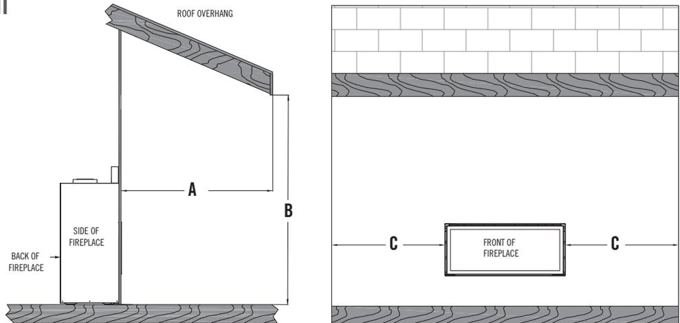
The overhang (A) must be a minimum of 1/2 or greater of the roofline elevation (B) above the base of the fireplace.
