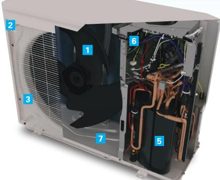
Inverter Board Cooled by Refrigerant Circuit<sup>1</sup>. Elimination of condenser fan pressure drop caused by heat sink used on previous generations.
